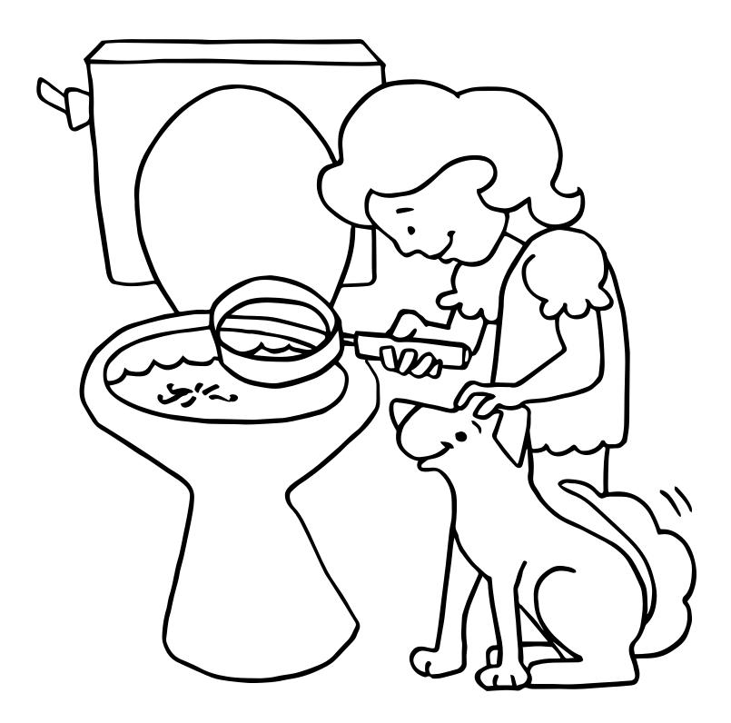
Have a parent help you take the top off the tank at the back of the toilet. Place a few drops of food coloring in the tank. If the color shows up in the bowl, you might need a new flapper. Don't forget to flush after!
