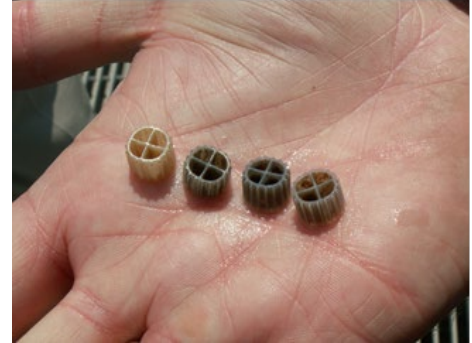
The IFAS process adds High Density Polyethylene media, as depicted here to the process basins.
