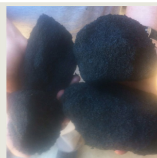
Figure 2: Scaling within a GAC vessel due to Calcium Carbonate Formation. Granular GAC has agglomerated into "soft ball" solid chunks which prevent full use of the adsorptive media surface area.
