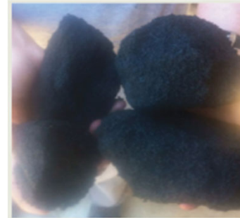
Figure 2: Scaling within a GAC vessel due to Calcium Carbonate Formation. Granular GAC has agglomerated into "soft ball" solid chunks which prevent full use of the adsorptive media surface area.
